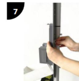
7 Tighten the two wing nuts at the rear side.
