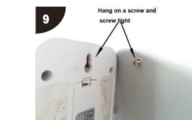
9 Hang the thermodetector onto the screws and tighten the wing nuts at the rear side.
