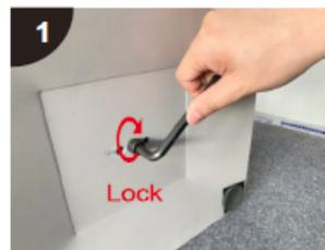
1 Use Allen Key to fix the screws on the base.
