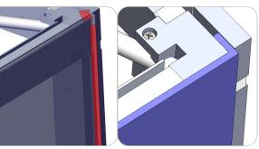
To apply the silicone edge graphic, start by pressing the SEG into the top left corner hub of the frame. Continue to press the SEG into the extrusion bar fabric channel. Keep pressing the SEG into the bar fabric channel until you make down to the bottom right corner hub of the frame. This also works for the second printed graphic option on the back side of the frame when horizontal channel bars are installed.
