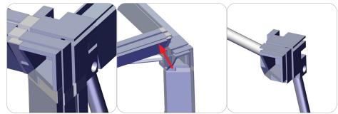
To remove the channel bars, start by pulling the end caps off the corner hubs.
