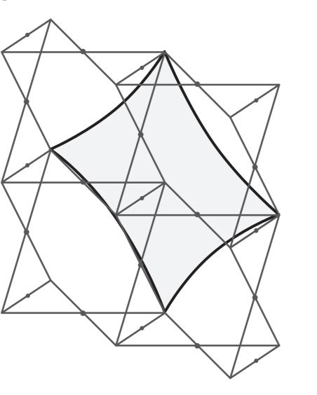
X-FACTOR: A term describing the result of tension at all corners and connection points of an Xpressions skin when placed on a frame. The artwork will be stretched with the least amount of distortion at the center of each quad, and the most distortion within the outer 3-5" of the skin. It is not a live area, as the image will be visible.
