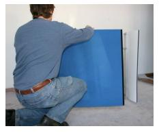
5. Go to the side of the counter with velcro on the top and bottom edges. This is the side that will have the solid panel. Velcro the solid panel into place with the additional velcro showing on the sides.
