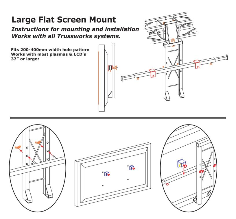
Mount bracket to truss, using the horizontal or vertical bracket provided for your application.
