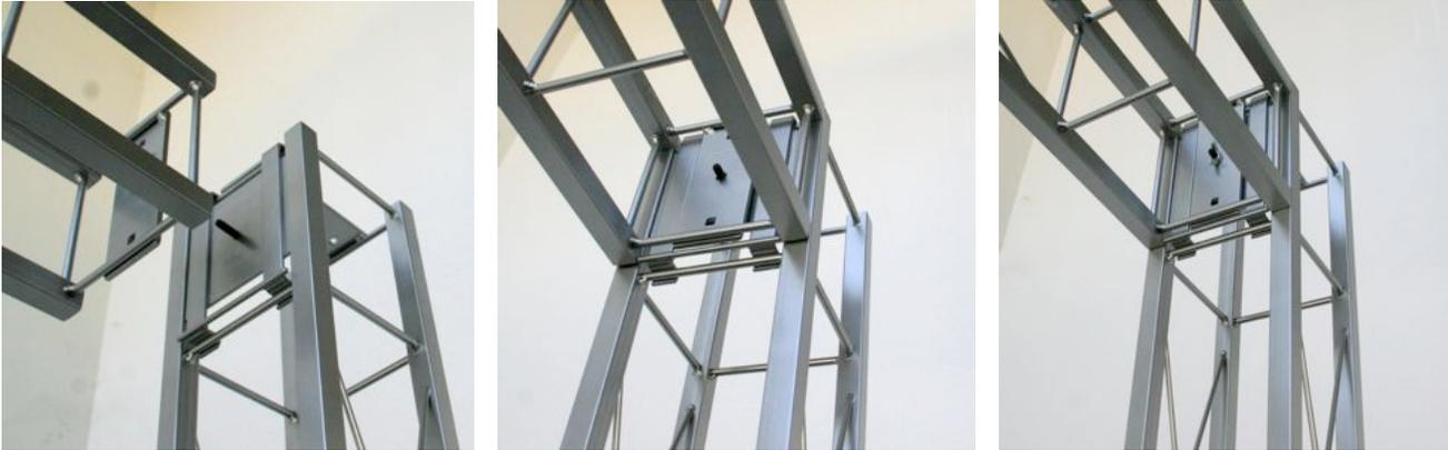
Hang the bracket from the top wire with the bottom tabs behind the second wire. Position the horizontal such that the bracket stud goes through the center hole. Install and tighten the wingnut making sure the alignment wire goes between the Horizontal tubes. The horizontal should be flush with the top of the upright.
