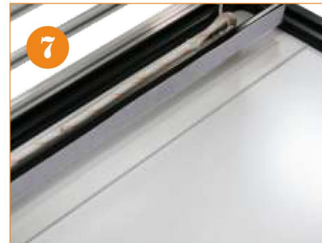
7. Attach the bottom aluminum bar's male to the velcro on the base
