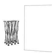
**WARNING!** DO NOT FORCE CLOSED. To avoid damage, all hooks must be disconnected before collapsing frame.
