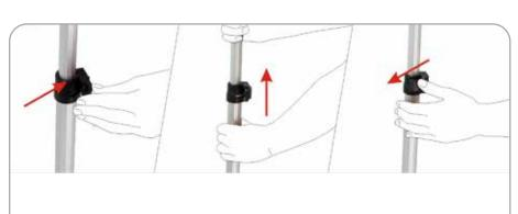
Open the latch of the telescopic pole and raise to graphic height. Close latch to secure.
