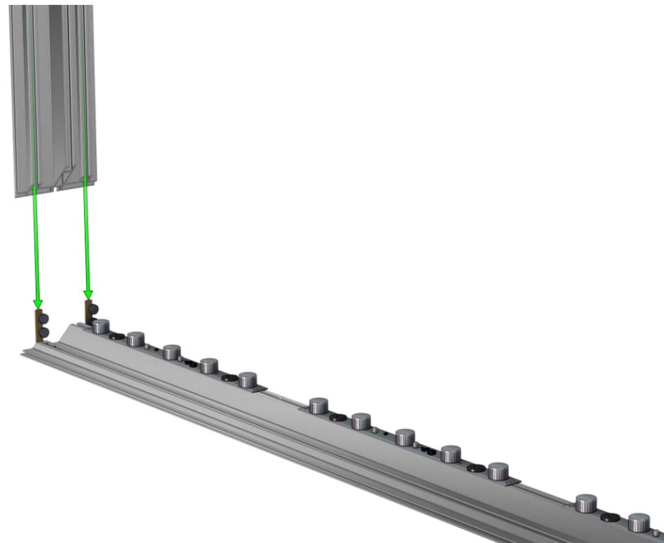
**2.** Join the two halves, and fasten with the thumb screws as shown.
