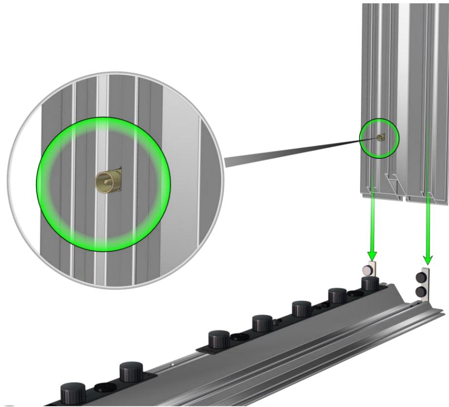
**7.** Next step is to take the center brace extrusion, and install it in the center of the display, directly over the seam where the two lower extrusions meet.
