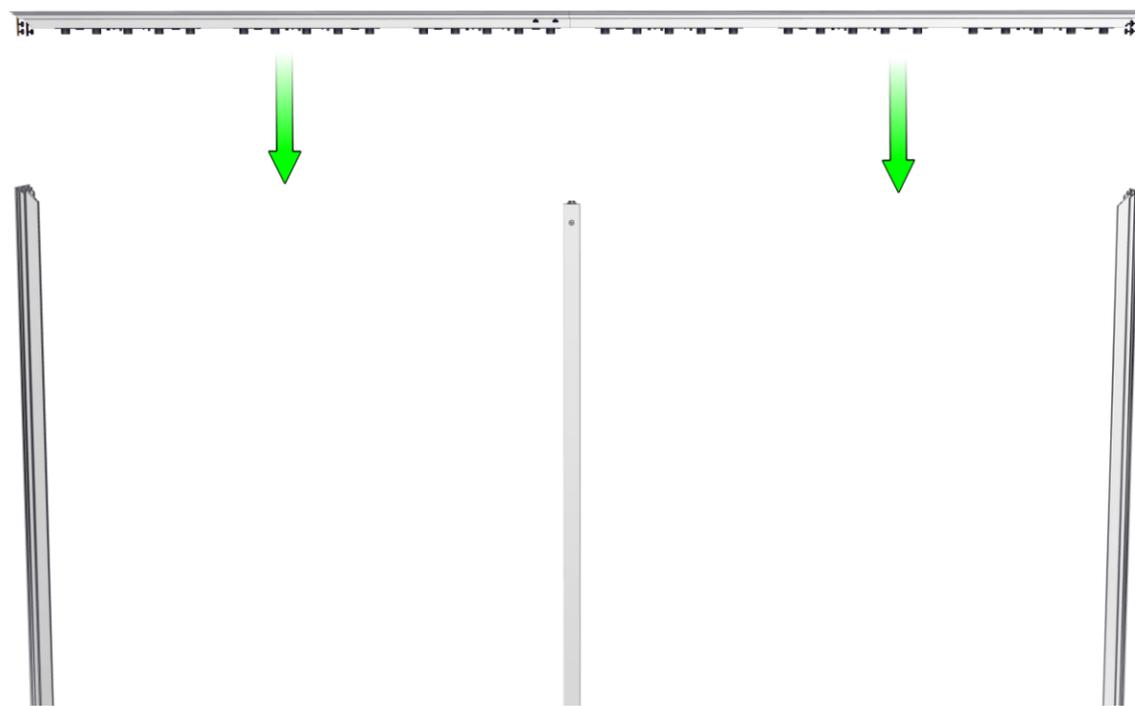
**10.** Secure extrusions with thumb screws as shown.
