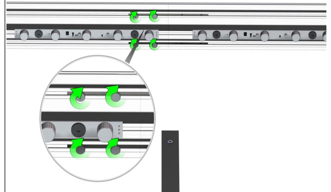
**12.** To secure the top assembly, fasten thumb screws as shown at all three locations.
