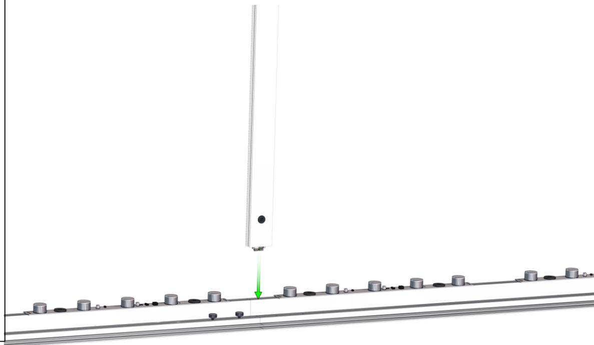
**6.** Secure extrusion with thumb screws as shown.
