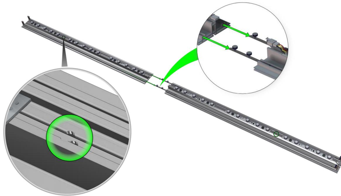
**3.** Next, take one of the vertical extrusions\* and install on left side as shown.
