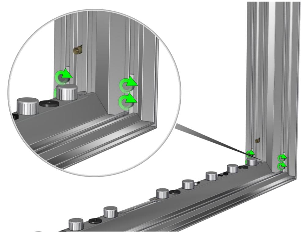
**8.** To secure the center brace turn one half turn clockwise with the provided tool.\*
