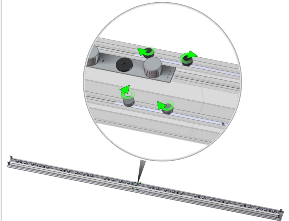
**4.** Tighten all four thumb screws as shown.
