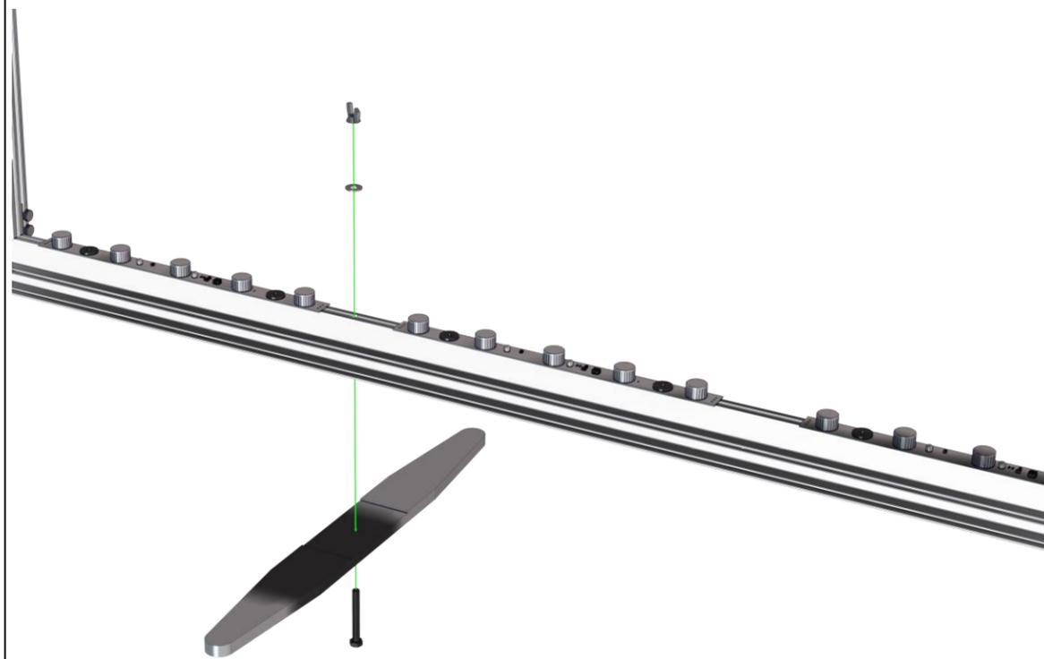
**14.** Secure feet by tightening the wing nuts firmly.
