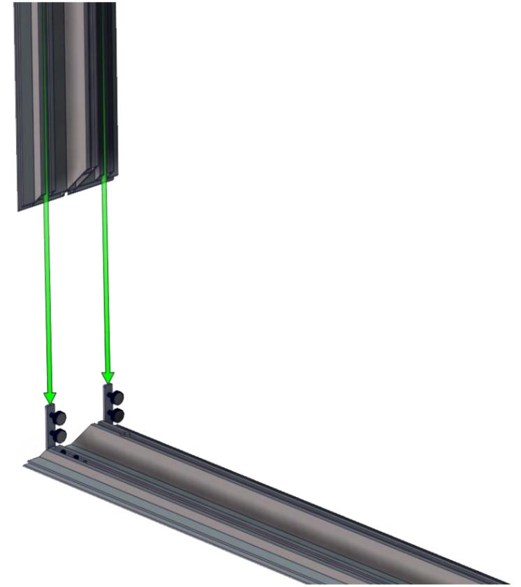
4. Next step is to take the 8' vertical section **with** lights and install it over the brackets as shown.
