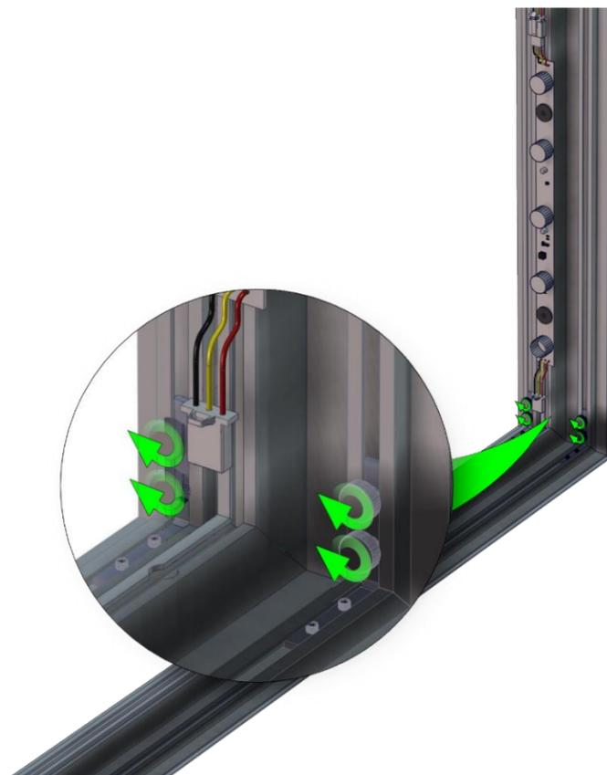
**7.** To secure, tighten all thumb screws until tight.
