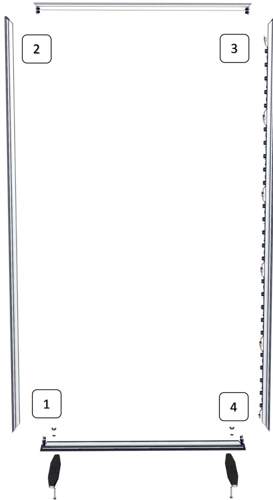
1. Begin with the lower extrusion signified by the holes for the foot bolts as highlighted.
