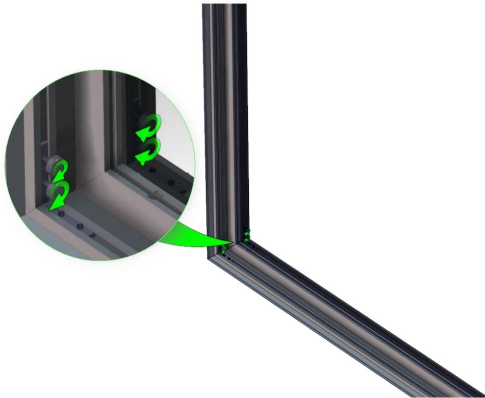
2. Next, take the 8' vertical section with **no** lights, and install over brackets as shown.
