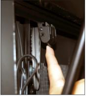
4.Attach monitor to mount on tower and secure it with clips on the back of monitor mount portion.
