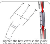
Tighten the hex screw so the joiner seperates and tightens against the inside of the tubing, locking the joiner and tubing together.
