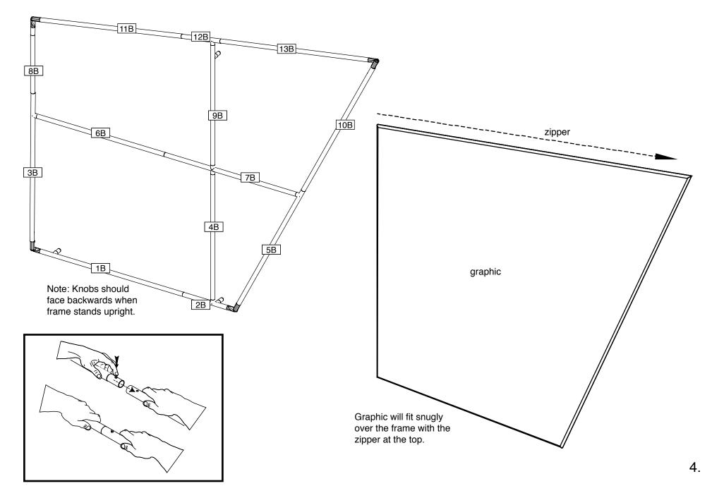
Step 4. Attach foreground frame to background frame Attach two units together using 14B, 15B and 16B.
