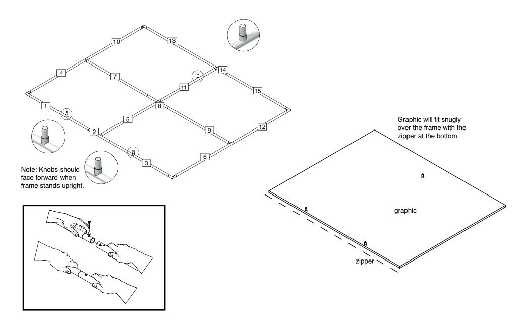
Step 2. Attach feet to background frame using details shown below. Stand unit upright. Adjust the height of feet to ensure display is level.
