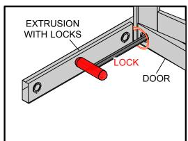
Step 2. Lock left and right VE-36 posts to bottom VE-32s using detail below. Slide VE-45s into VE-36s.
