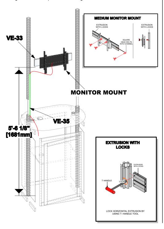
Step 6. Attach standoffs to VE-36s using attachment detailed below. Attach wings to standoffs.
