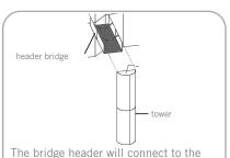
back wall using the same assembly in step 9. To attach to the tower, slide the header bridge into connectors halfway and tighten. This will prevent the panel from sliding down the channel.
