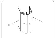
To assemble the counter start with the left panel working towards the right until all counter panels have been connected.
