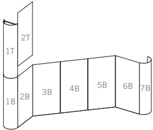
Add the first panel marked 1T (1 Top) into position. Add the second panel, 2T (2 Top) by sliding the aluminum link into the routed portion of panel 1T. Slide panel into position. **5**
