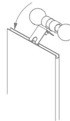
Position light fixtures where indicated on the panel by placing the lights into the channel and lower down. **7**
