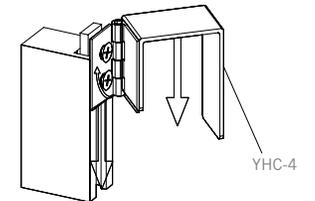
To assemble the header, attach the separate pieces together with the sliding connectors top and bottom and tighten the thumbscrews. The hinged connectors on the sides of the header hook over the panels as shown on page 2. **8**
