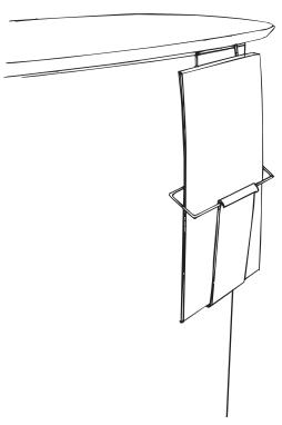
4. Install the top, skirting board and graphic wrap on the Expand PodiumCase. Now you can hang the Expand BrochurePocket from the bracket. Choose the left, the right or both sides!
