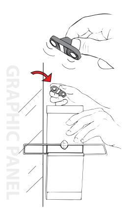
3. Use the supplied super-magnet(s) to attach the Expand BrochurePocket to the graphic.
