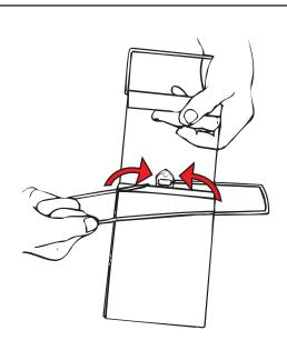
1. Install the metal retainer into the holes on back of the clear plastic pocket.
