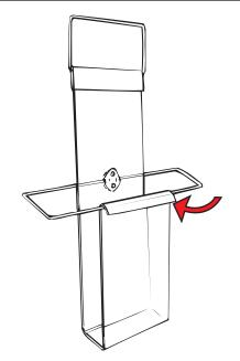
2. Hook the metal retainer over the outside portion of the plastic pocket.
