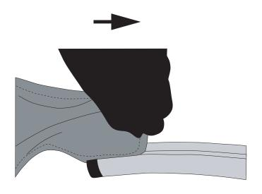
Insert end of new graphic into the groove and slide into place\*.
