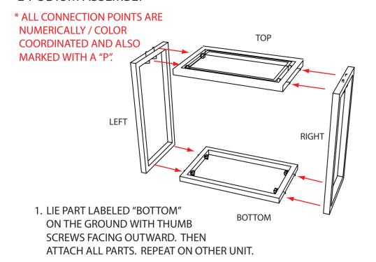
2. ATTACH COUNTER TOP SUPPORTS TO THE THUMB SCREWS ON THE "RIGHT" AND "LEFT" PARTS.
