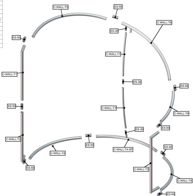
**C-WALL FRAME ASSEMBLY:**Assemble unit by laying tubes flat on the floor. Connect the tube rails following the labels by matching number to number.
