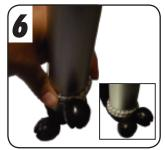
Push down on the white bungee, securing the black bungee between the base of the pole and the stand bottom. Set-up is complete.
