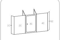
To assemble the counter start with the left panel working towards the right until all counter panels have been connected.
